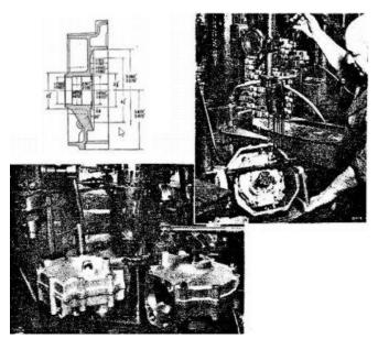
After both crankcase halves are ready, they are put together with four bolts in order to mill the mounting for the machines that still use a separate dynamo. The photo in question clearly shows how the crankcases are secured to the work table and between the two crankcases we see the guide for the cutter. About 3/32" of aluminium is removed from both crankcases at the same time, in a time of 1 minute and 33 seconds.
