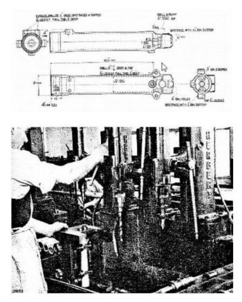
In addition, the entire slider is brought to a 1 9/16" diameter over a length of more than 10". The slider is first pre-rotated, then accurately turned and then the reamer goes through. In these three operations, the turret remains in the same position and the tool must therefore be able to be changed quickly. A laborious stage and the entire cycle takes no less than 11 minutes.
